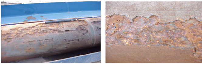
Fig. 1. Examples of severe localized corrosion of electric submersible pump motor casing.
